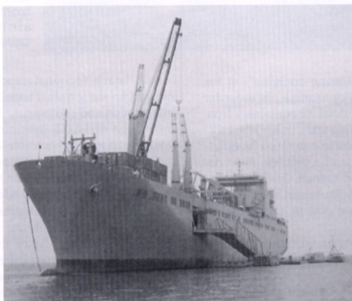
□ A logistics support vessel uses a roll-on-roll-off discharge facility to transfer equipment from its cargo hold to lighterage alongside.
