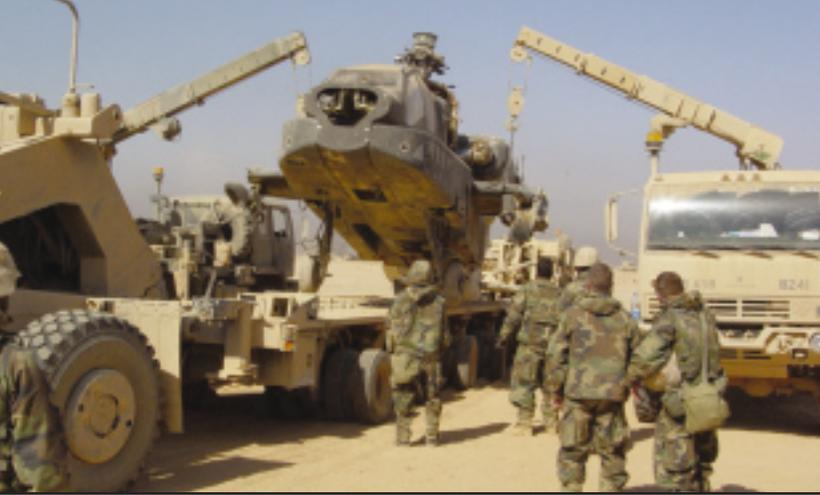
*Two wreckers are used to recover a crashed AH-64D Apache Longbow helicopter.*
