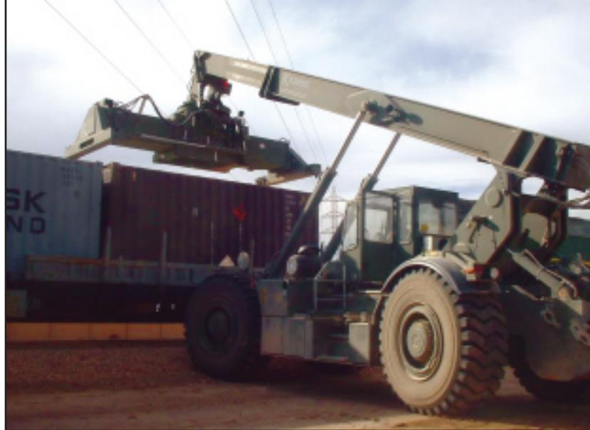
*A rough-terrain container handler is used to offload containers of bottled water from railcars at Al Iskandariyah, Iraq.*
