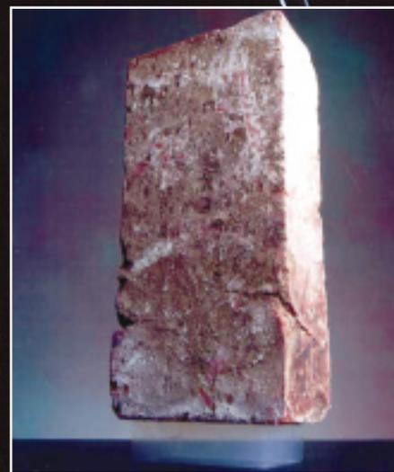
*Aerogel is 99.38 percent air (on page 25), but it can hold 4,000 times its own weight (for instance, the brick above) and act as a heat barrier (at left, protecting crayons from a torch).*
