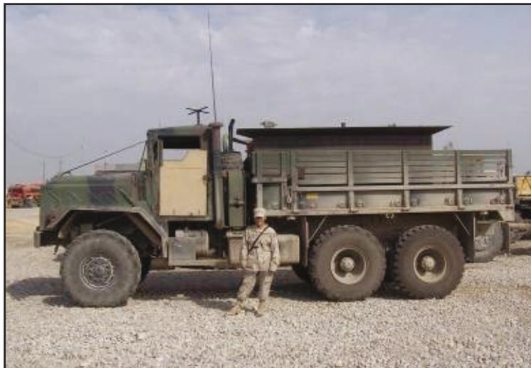
*This M923 5-ton cargo truck has been augmented with armor on the driver's door and a gun box in the truck bed.*
