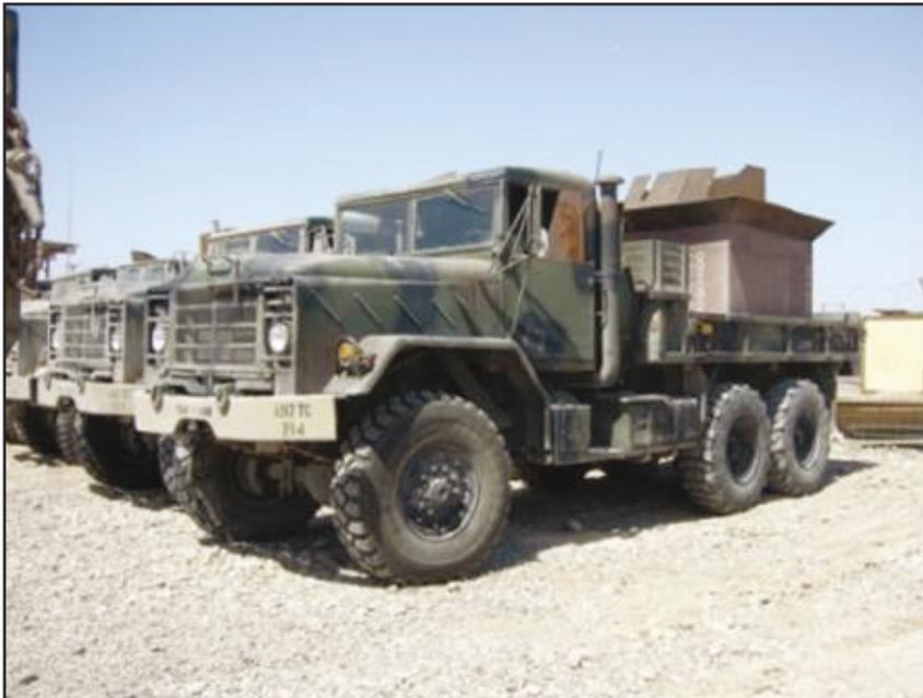
***The maintenance section of the 497th Transportation Company continuously updated the gun box design on their gun trucks. These trucks have a four-post ring mount and a fully enclosed shield for the gunner.***
