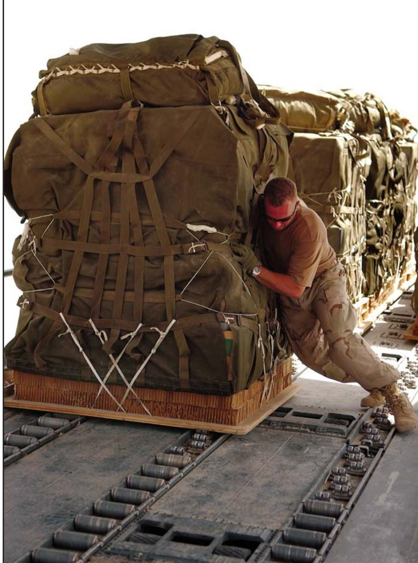
*A member of the 173d Airborne Brigade in Vicenza, Italy, loads 12 Container Delivery System bundles onto a C-130J aircraft for an equipment drop at an undisclosed location.*
