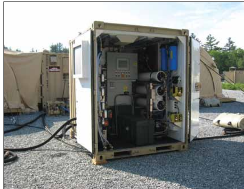
The shower water reuse system is being used at forward operating bases to reduce the need for water resupply.
