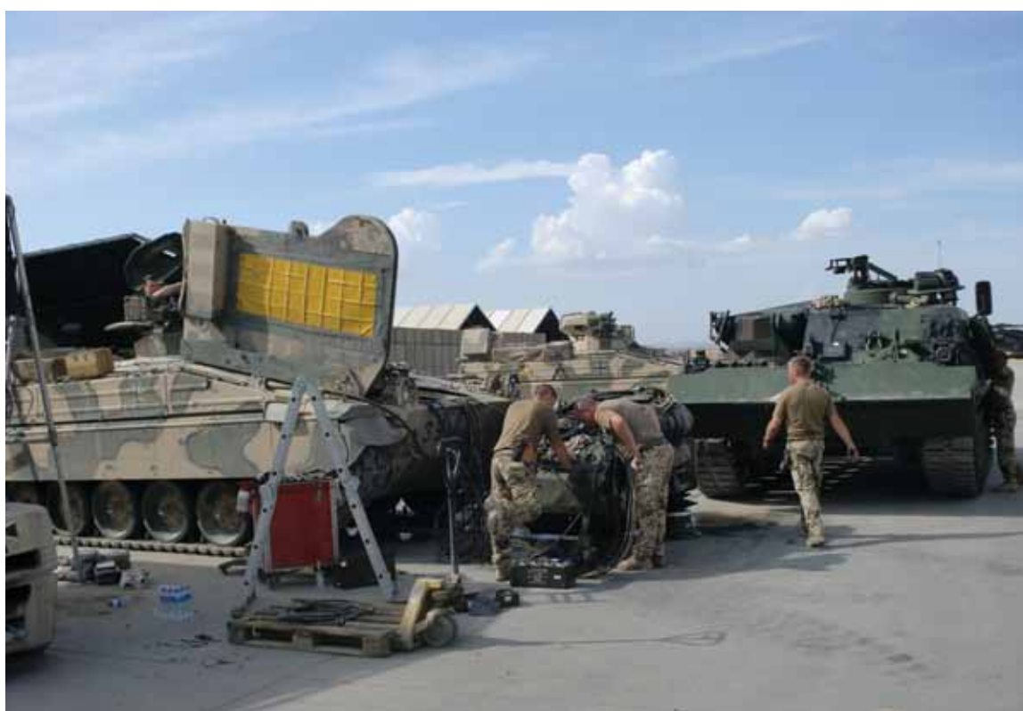
German military mechanics change the engine of an armored infantry fighting vehicle at a provincial reconstruction team logistics base in Afghanistan.
