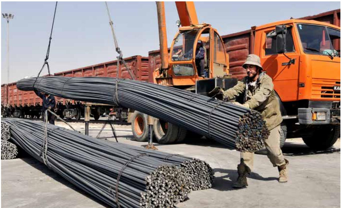
*Steel rebar, imported through Uzbekistan, is guided into place after a crane lifts the rods out of a railroad gondola car at Rail Port 4, Niababad. After offloading the rebar from the railcar and staging on the loading dock, the rebar is then lifted onto trucks for transportation to construction sites around Afghanistan. (Photo by Sgt. 1st Class Timothy Lawn)*
