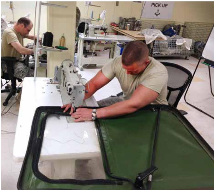
*A Soldier repairs tears on a humvee door using a long-arm sewing machine.
