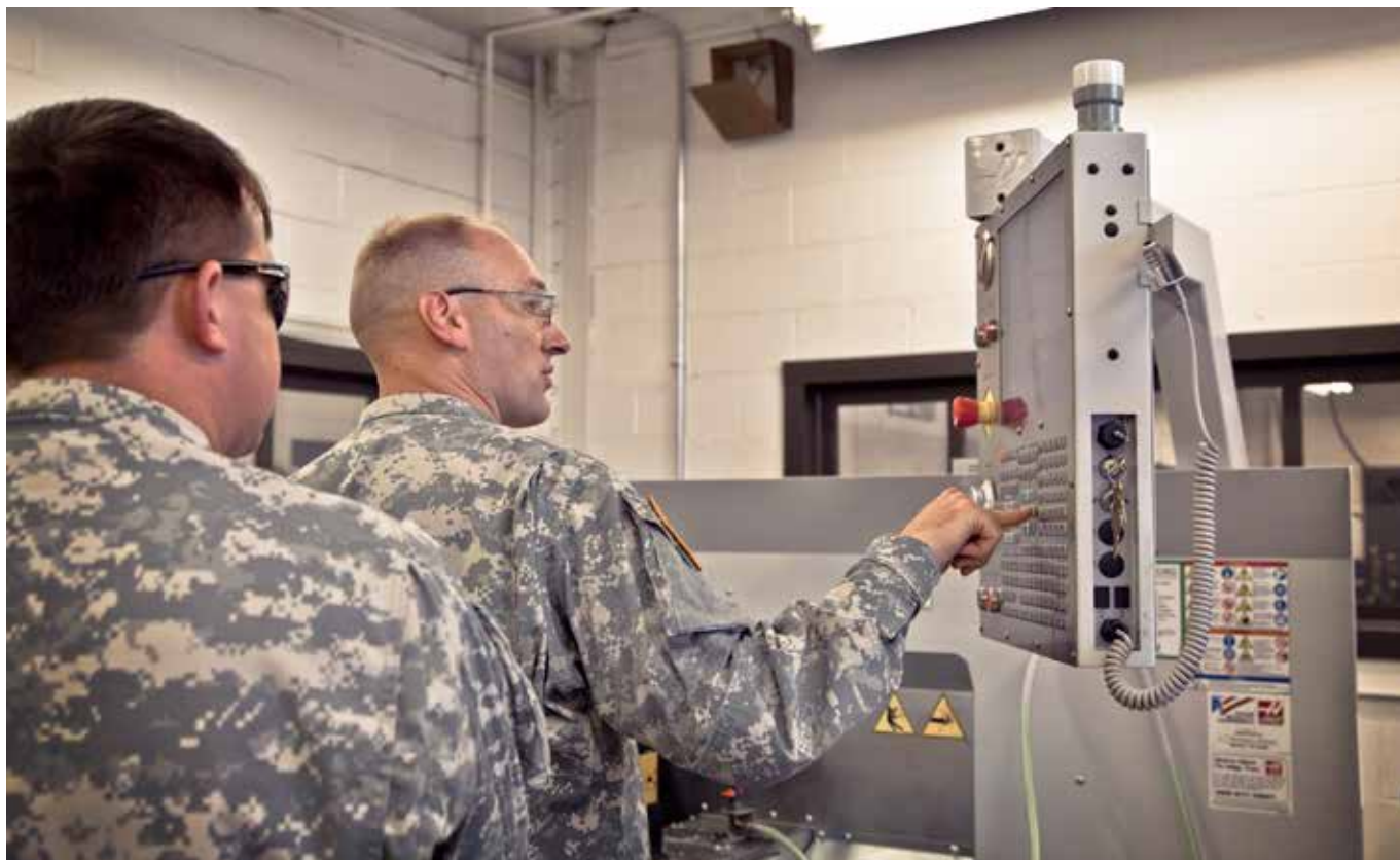
Soldiers from B Company, 181st Brigade Support Battalion, 81st Brigade Combat Team, Washington Army National Guard, train on the Haas Automation TL-1, a computer numerical control lathe, at the Sustainment Training Center at the Camp Dodge Joint Maneuver Training Center in Johnston, Iowa.
