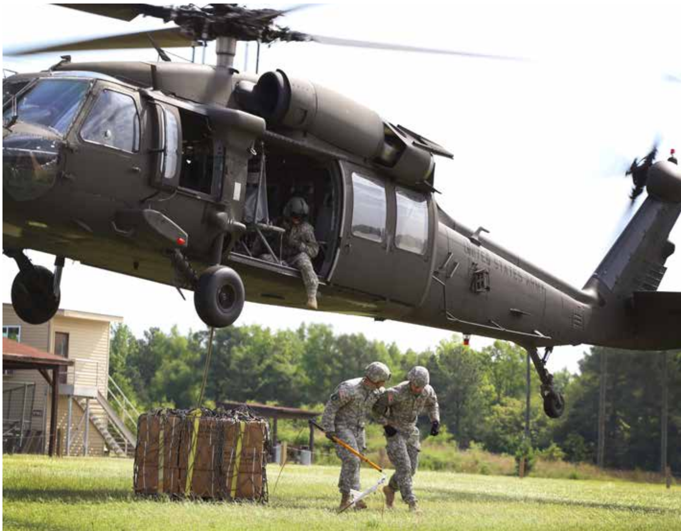
A noncommissioned officer instructor trains a Basic Officer Leader Course student in properly attaching a sling load to a UH-60 Black Hawk helicopter. This training teaches students the capabilities of aerial resupply and how it can be used across kinetic operations. (Photo by Adam Gramarossa)
