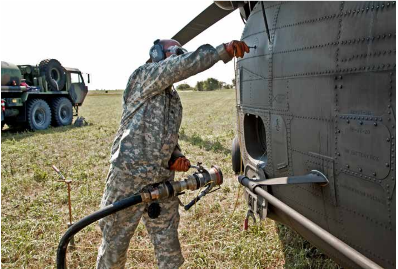
A distribution company Soldier trains on the heavy expanded-mobility tactical truck tanker aviation refueling system at the Army National Guard's Sustainment Training Center.
