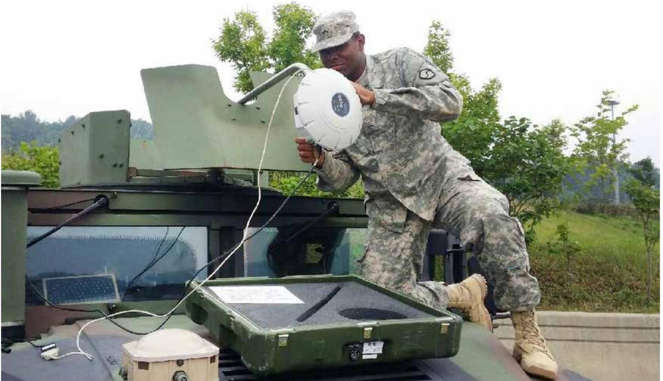
*A transportation management coordinator Soldier from the 665th Movement Control Team makes adjustments to a Portable Deployment Kit interrogator installed on his crew's humvee. The interrogator is used to provide in-transit visibility of radio frequency identification tags attached to a convoy's vehicles and equipment. (Photo by 1st Lt. Carlos Moreno)*
