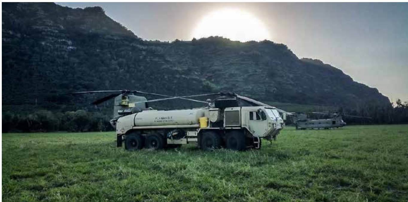
Soldiers from Echo Company, 2nd Battalion, 25th Aviation Regiment, conduct a cold refuel of a CH-47 Chinook helicopter during Lightning Forge in February 2016 on the Hawaiian Islands. (Photo by Cpl. James Halstead)
