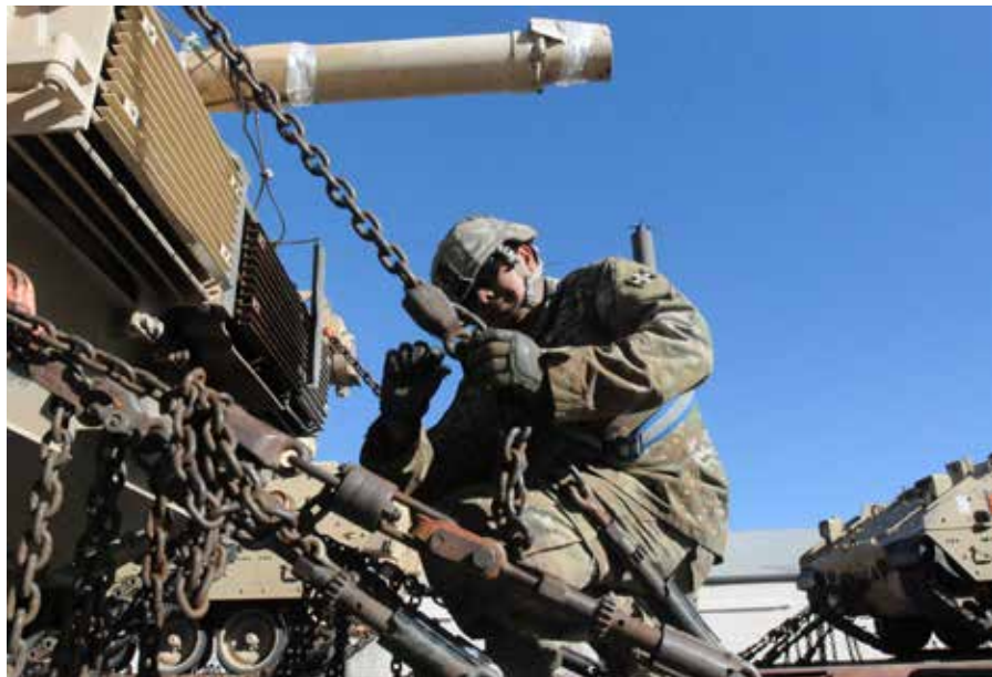
Beginning his unit's move to Poland for Operation Atlantic Resolve, an M1A2 Abrams crewman from the 3rd Armored Brigade Combat Team, 4th Infantry Division, secures a tank after it is loaded onto a rail car at Fort Carson, Colorado, on Nov. 15, 2016. (Photo by Ange Desinor)
