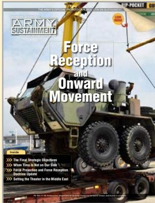
*A crane lifts a heavy expanded-mobility tactical truck onto a flatbed during port operations at Busan, South Korea, on July 13, 2017. This marked the first time the 35th Air Defense Artillery Brigade received air defense missile equipment by sea in order to integrate it into the air defense architecture on the Korean Peninsula. (Photo by Capt. Jonathon Daniell)*
