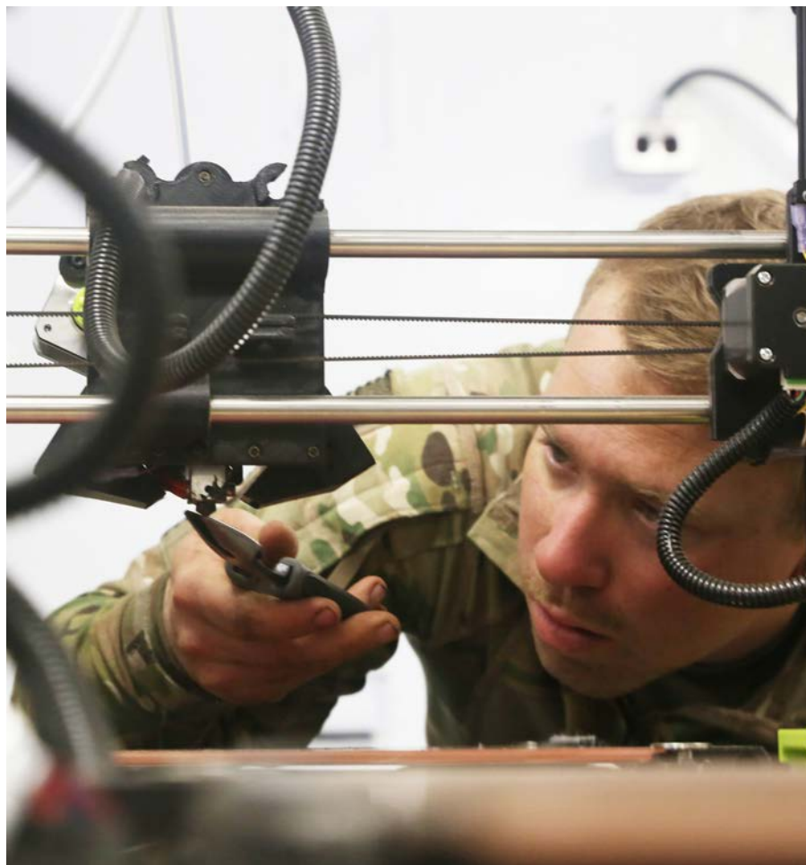
Pfc. Jimmy Roe fixes a 3-D printer that is part of an expeditionary system called the Rapid Fabrication via Additive Manufacturing on the Battlefield at Amberg Training Area in Amberg, Germany, on May 4, 2018. (Photo by Spc. Elliott Page)
